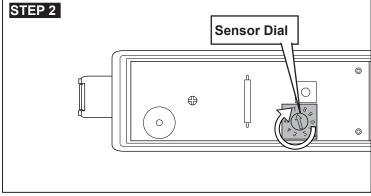
**NOTICE** ALWAYS confirm functionality of the vibration sensor after any changes or adjustments are made. Refer to Installation STEP 6 to test the vibration sensor operation.
