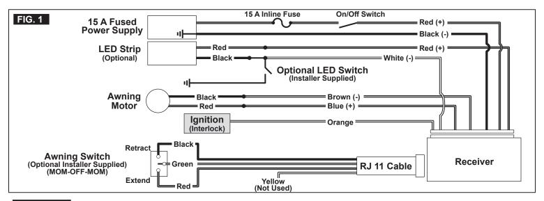
**AWARNING** FIRE OR ELECTRICAL SHOCK HAZARD. For all wire connections, use only NEC-approved connectors and terminals that are appropriately sized for the wire gauge. Failure to do so could result in death or serious injury.
