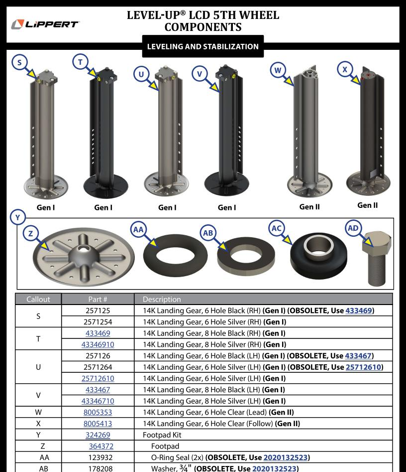
**NOTE:** A second O-Ring seal needs to be used above the footpad to secure kit. Rev: 09.18.23 Web: - <u>https://support.lci1.com/documentation/</u> - Ph: 432-LIPPERT (432-547-7378) - Email: <u>customerservice@lci1.com</u>
