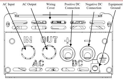
Figure 8 Electrical Connections Side View
