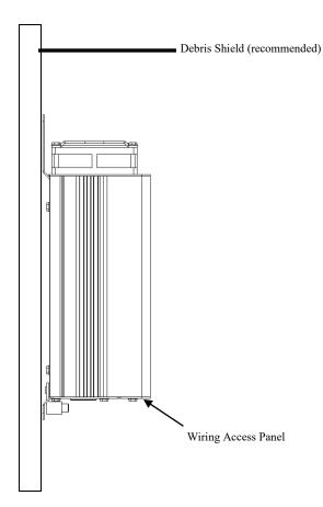
Figure 5 Vertical Mounting Configuration
