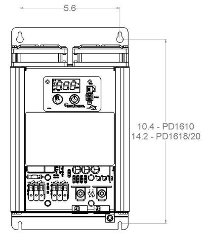
Figure 7 Inverter Mounting Hole Pattern
