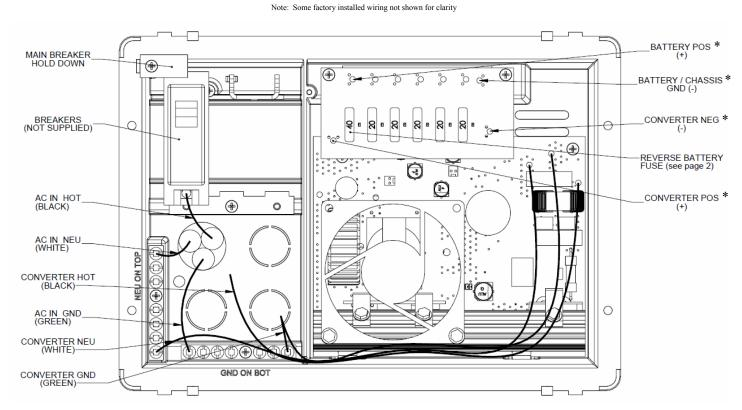
**Detailed Wiring Diagram**
