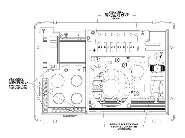
If you should need to replace the power converter for any reason, follow these steps to safely remove the converter section.
